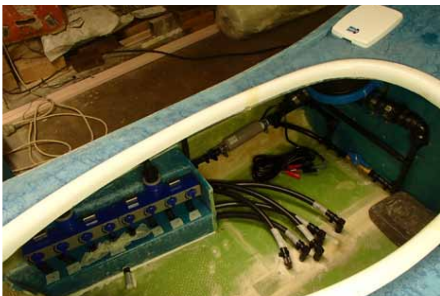
Tap control panel – one tap per chamber. This array is duplicated in the vestibule of the pod (pic: Richard Barnes)
